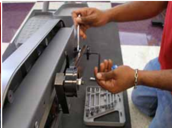
Fig. 8: installing the new control link assembly
